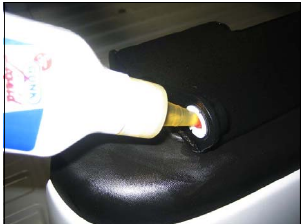
Put a drop of machine oil on each nyliner at the initial installation. This helps the nyliner seat and polish for a long life.
