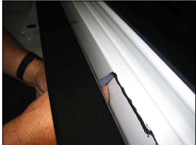
Pull the headboard rail back, and run a bead of RTV sealant across the inside of the truck headboard.
