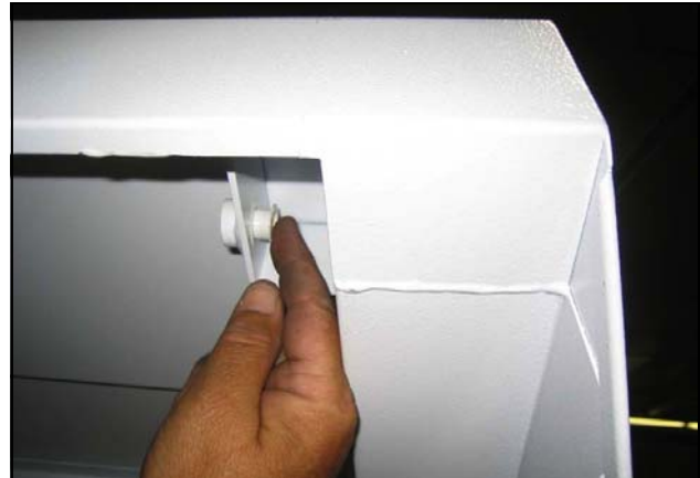
Install a nyliner inside the front corners of the cover. The shoulders of the nyliners must be toward the outside of the cover. Put a drop of oil on the nyliner.
