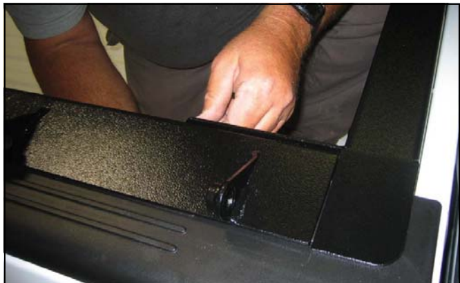
Make sure the bed rail is tightly fitted at its front edge to the headboard rail. Tighten the 5/16” bolts.
