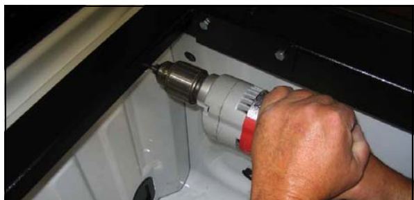
Drill three 1/4" holes on each side.
