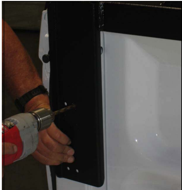
Drill a 5/16" hole through one each of the top and bottom holes in the bed mounting rail.
