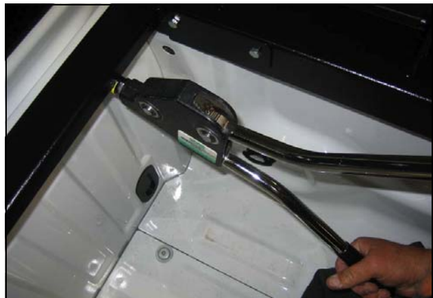
Install three 1/4" steel rivets on each side of the headboard rail. Do not use aluminum rivets.
