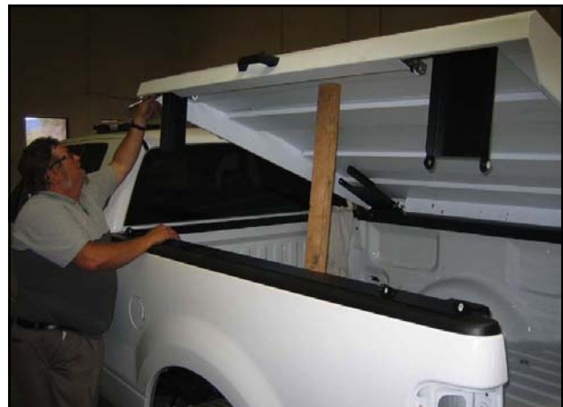
Install the upper leg assembly with the concave sides facing out. Wrench the 1/2"-13 x 2-1/2" bolts into where they are bottomed out.
