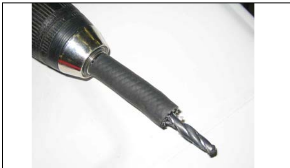
Slip a piece of hose over the drill bit to keep it from hitting the back of the cab.
