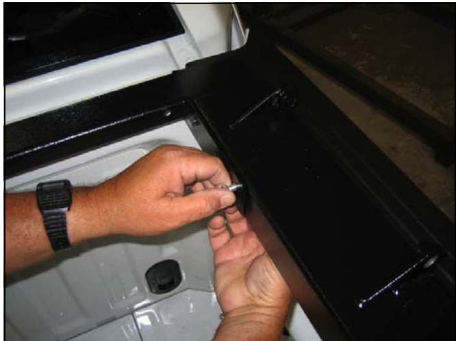
The bed rails fit on the outside of the mounting ears on the headboard mounting rail. Install the 5/16”-18 x 3/4” bolts and nylock nuts.
