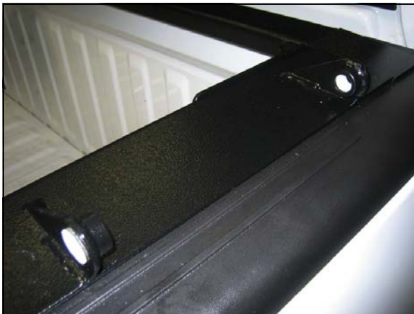
Install nyliner bearings in the mounting clevises. The shoulders of the bearings go on the outside of where the legs bolt in.
