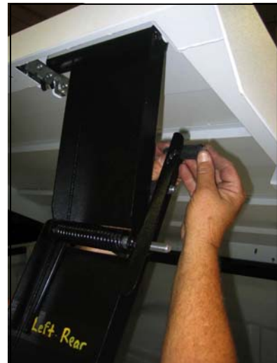
On the rear legs only, install a stop assembly on the long arm as shown. This engages the “Z” bracket inside the cover.
