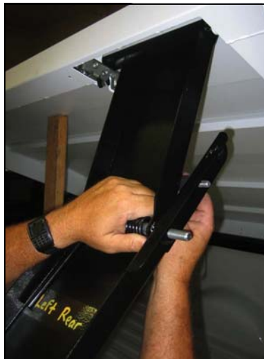
Rotate the lower leg around against the spring pressure and install a stop assembly as shown.
