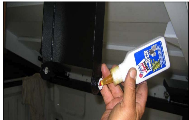
Install nyliners into the lower tubes in the legs, with the shoulders facing outward. Oil the nyliners.
