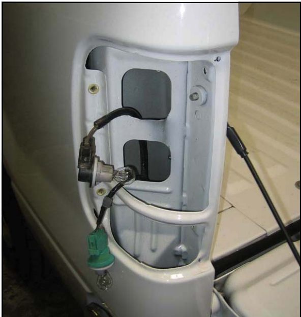
Remove the tail lights and determine the best places to drill the holes. Leave the tail lights out for now.
