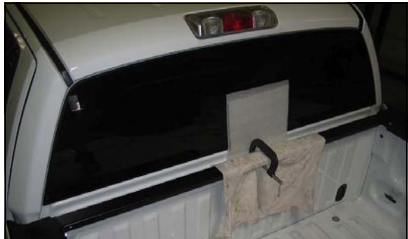
With the headboard rail centered, clamp it into place.
