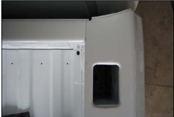
Make sure the headwall is not broken out of position. Correct any alignment problems before proceeding.
