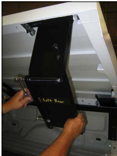
Assemble the spring sleeve, torsion spring, 10-inch bolt and legs as shown. Wrench the bolt into where it bottoms out.
