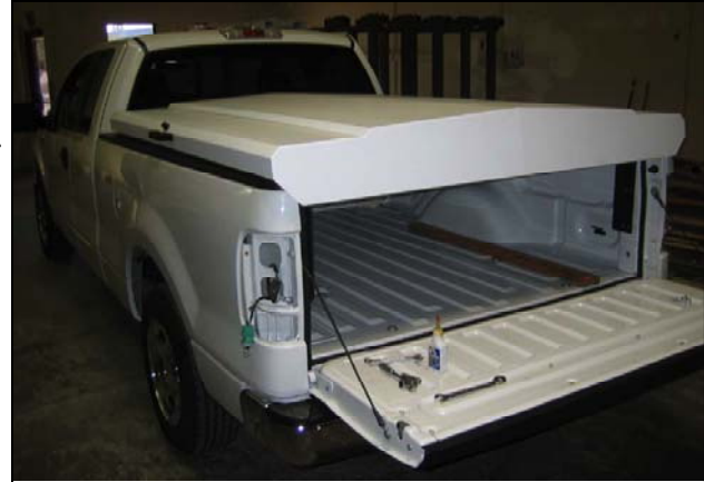
With the tailgate down, place the cover onto the truck. Note that the tail lights are still removed.
