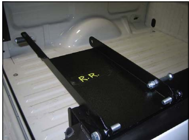
Install the lower right legs as shown. Leave them extending over the inside of the truck bed.
