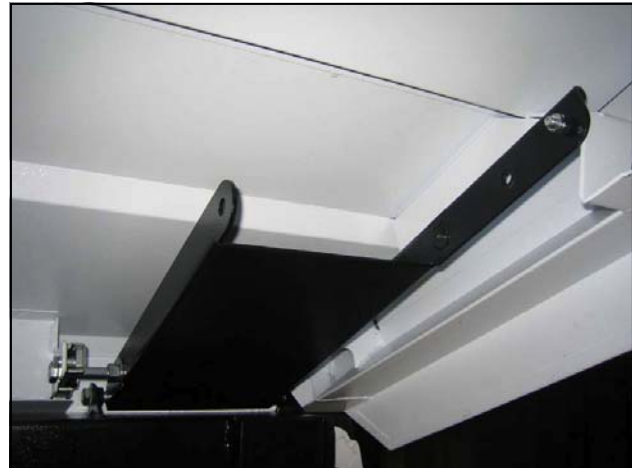
From the inside of the bed, lift the rear of the cover (or have a helper lift from the outside). Get the long arm of the right rear leg above the “Z” bracket (on the far right). Make sure the striker bolt is latched in the rotary latch of the cover (on the lower left).
